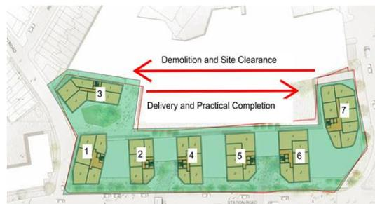
Figure 10.4.3 Indicative construction sequence for the Station Road Offices Site.
