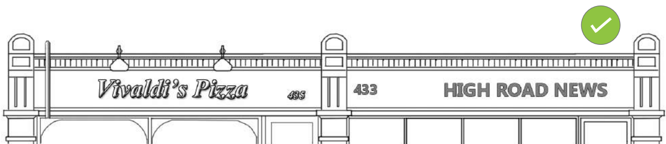
Picture 64. Fascia Signs
