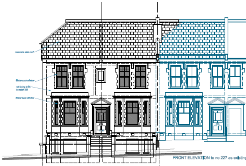
Terrace Extension / Front Elevation to Archway Road
