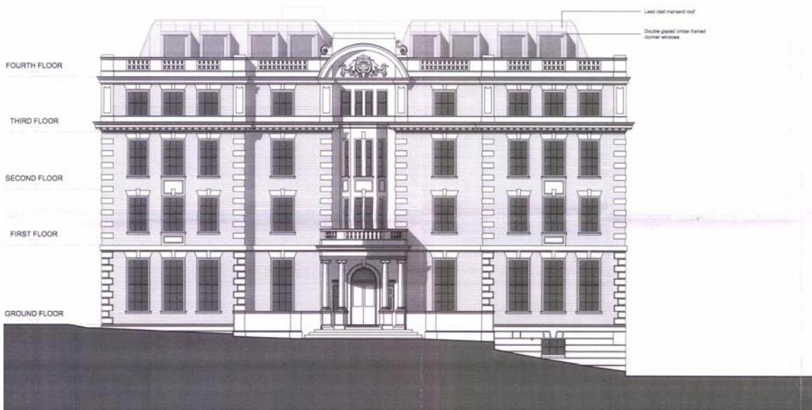
Proposed Front Elevation (Showing roof addition)
