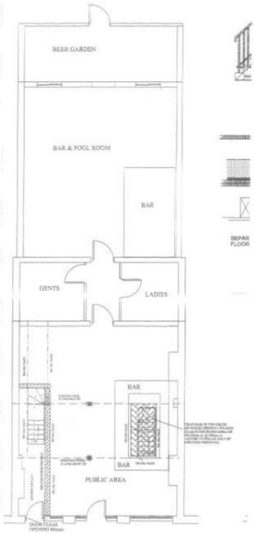
GROUND FLOOR PLAN AS PROPOSED-PUBLIC BAR
