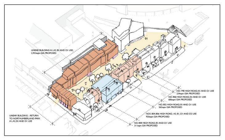
Axonometric sketch showing proposed 'Linear Building' and refurbished and extended High Road buildings
