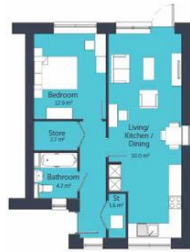
1B2P Flat Layout - 60.0 m 2 - Type 1 Ground Floor
